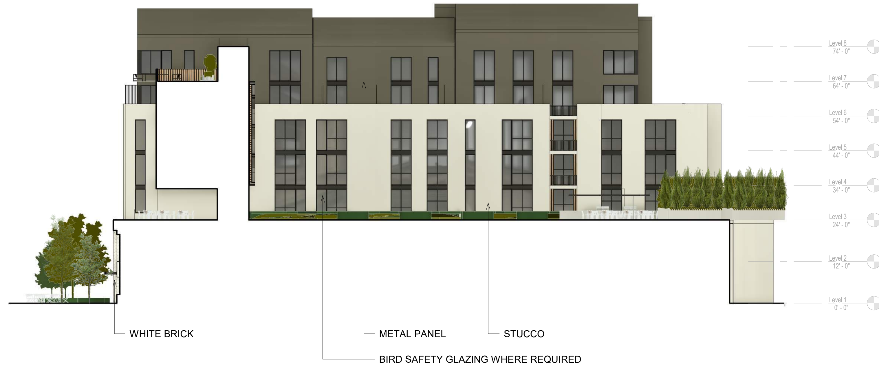
3 COURTYARD ELEVATION South-West Scale: 1/16" = 1'-0"
